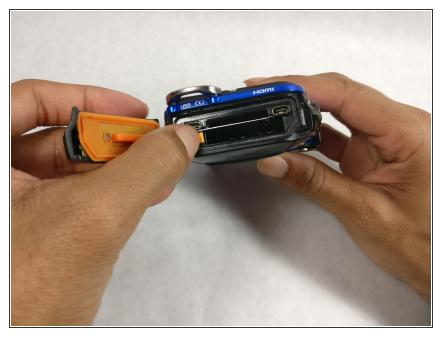
• Pull the orange tab towards the hinge to release the battery.
