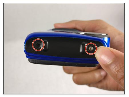
Unscrew two 4.0mm long hex head screws with a hex 1.3 screwdriver bit.
