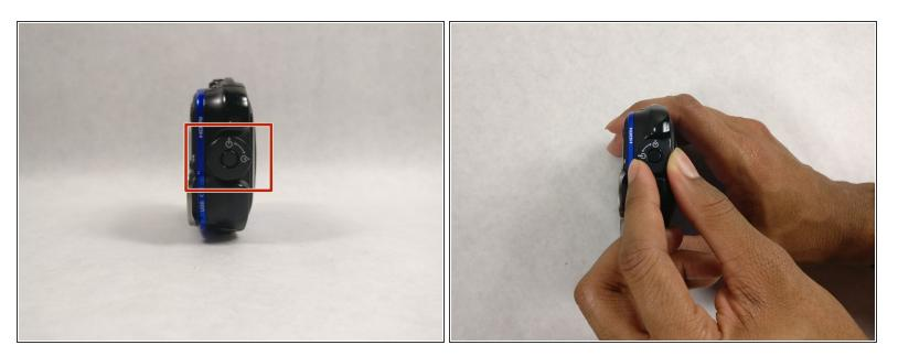
Push down on the center button and turn the dial on the side counterclockwise to open the battery compartment.
