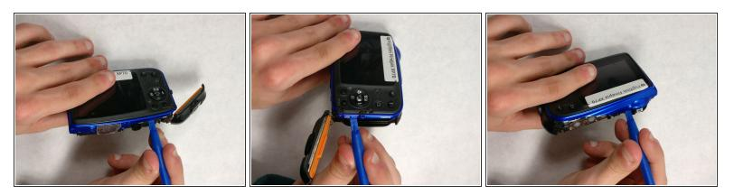
• Pry the back plate off with a plastic opening tool
