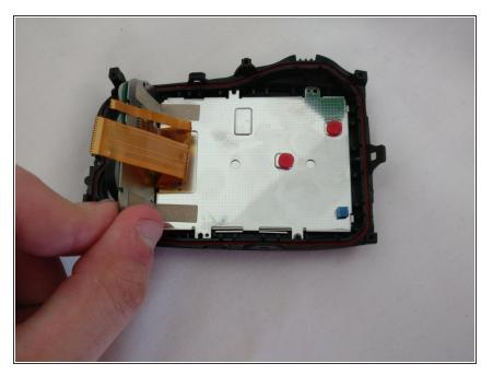
• Lift of the metal panel using a plastic opening tool.
