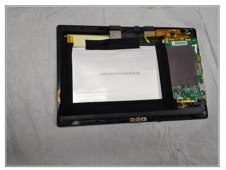
• Start by turning the tablet over with the screen down. Carefully use a plastic opening tool to pry the cover off. Start from the corner opposite the hibernate button.
