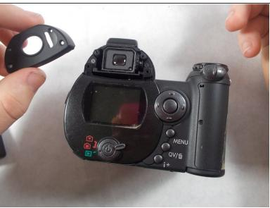
• Use a screwdriver to remove the four viewfinder cover screws.
