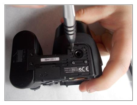
Remove 6 screws on the bottom panel.
