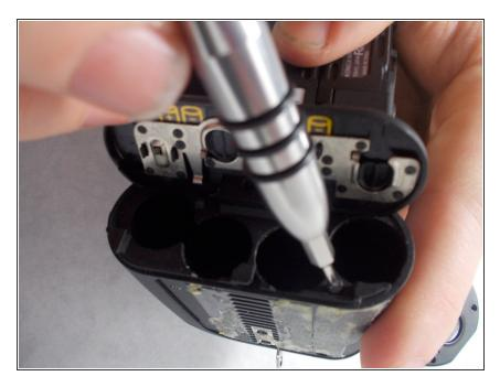
Remove 1 screw inside the battery chamber.
