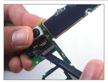
Using a spudger, lift up the metal connecting piece.
