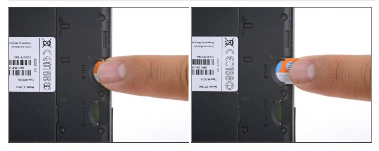
Slide out and remove the SIM card.
