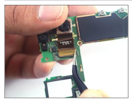
Using <u>tweezers</u>, remove the yellow film connecting the motherboard to the rear camera.
