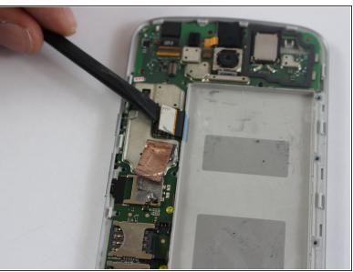
Using a spudger, remove the two metal pieces connecting the motherboard to the front casing.
