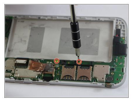
Remove two 4.0 mm T3 Torx screws connecting the motherboard to the front casing.
