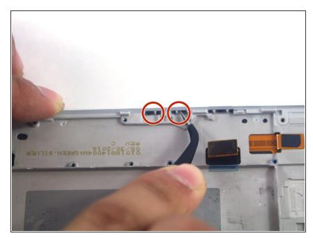
Using tweezers, remove the volume buttons.
