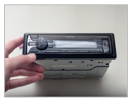
Press the eject button on the bottom left corner of the face plate.
