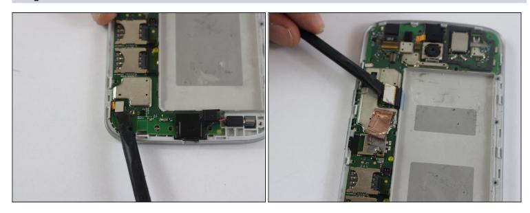
• Using a spudger, remove the two metal pieces connecting the motherboard to the front casing.
