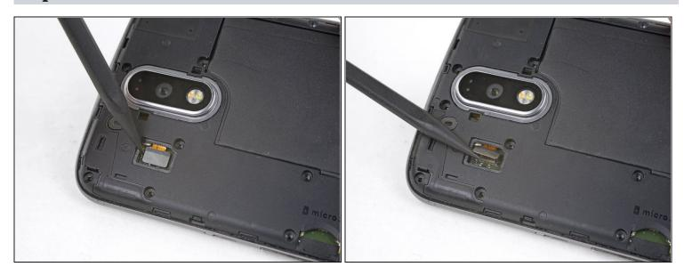
• Use the point of a spudger to pry up and disconnect the camera flash connector.
