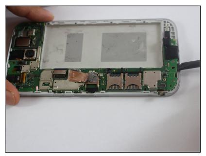
• Using a spudger, lift up and remove the motherboard.
