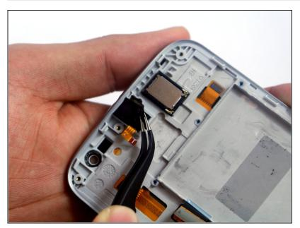
Using tweezers, lift up the black silicon piece covering the audio jack.
