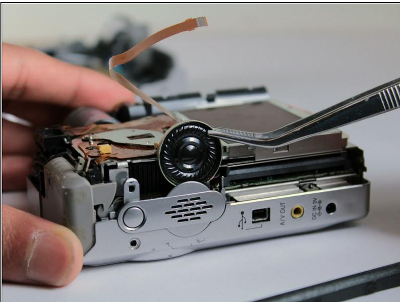
**⚠** Pull gently when removing the speaker so you don't rip the wire attached to it.
