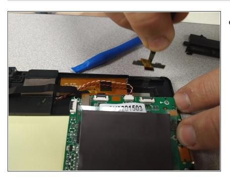
Using tweezers genitally pull up on the volume button board to remove.
