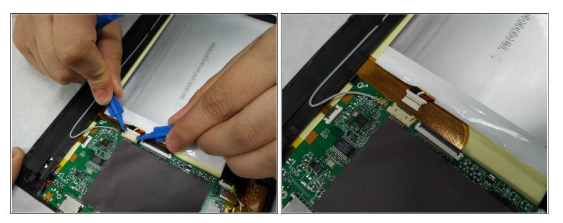
Using a small plastic opening tool; genteelly pull the connection off of the motherboard.
