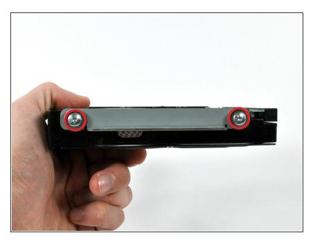
Remove the two 15 mm shouldered T10 Torx screws from the hard drive and remove the bracket.
