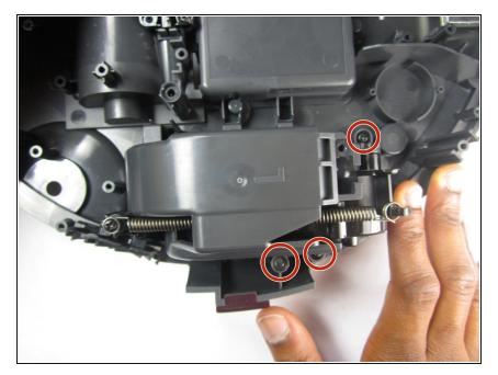
Remove three 10mm Philips #1 screws that are securing the wheel assembly.
