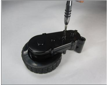
Remove the four 10mm Phillips #1 screws around the edges of the cover.
