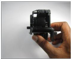
• Lift up on the plastic piece to remove the entire wheel assembly.
