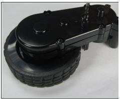
Remove the plastic frame by pulling outward on the two spots where it is fastened.
