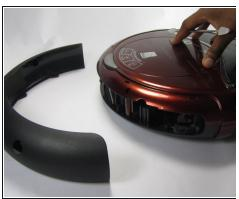
• Pry off the back bumper by going around the entire top of the bumper with the metal spudger.
