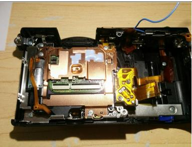
Open latches first. Gently remove both flex circuits attached to the image sensor. Take a note which one goes where
