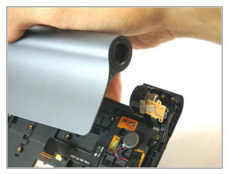
Lift and pull to detach the battery compartment.
