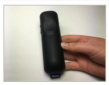
Place the remote control facing down on the table, so that the buttons are facing downwards.
