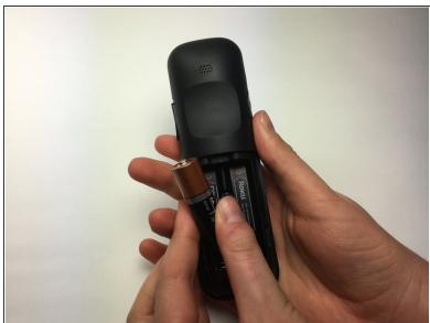
Remove the batteries from the battery compartment.
