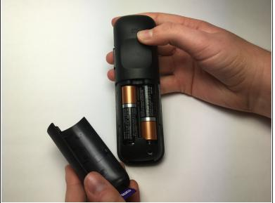
Remove the battery compartment cover from the back of the remote by sliding it outwards. This should reveal the batteries.
