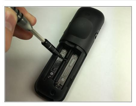
Turn the Phillips PH0 screwdriver counterclockwise to carefully remove the 6.9 mm screw located between both battery compartments
