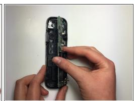
Using your right thumb, lift up on the left side of the motherboard to remove it from the bottom plastic casing.
