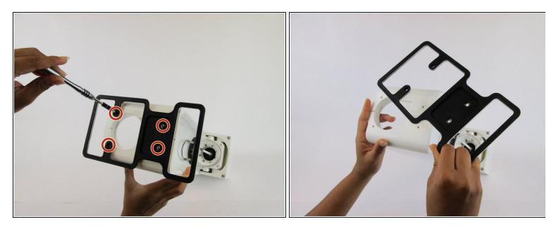
• Remove the four 17.8 mm screws from the bottom metal base using a <u>Phillips #1 screwdriver</u>.
