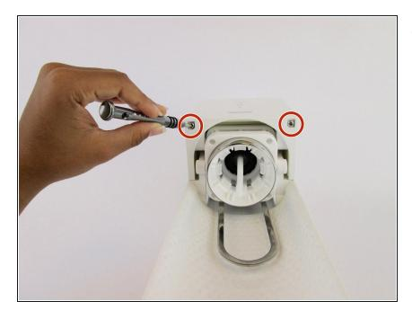
Remove the two 18.2 mm screws from the bottom of the front cover using a <u>Phillips #1 screwdriver</u>.
