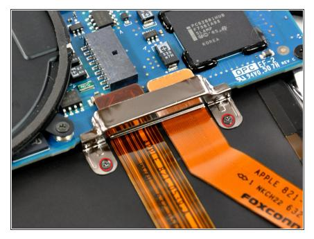
Remove the two small Phillips screws securing the logic board bracket to the upper case.
