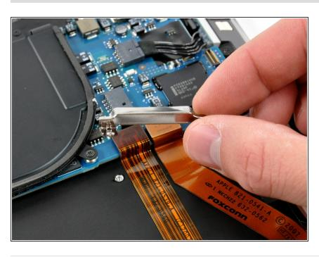
Lift the logic board bracket out of the upper case.
