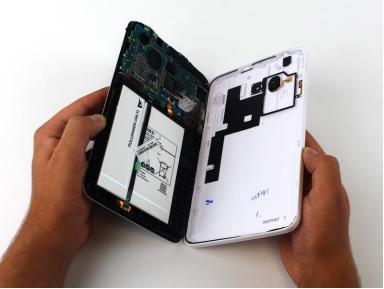
After separating the latches holding the screen and case together, slowly take the screen off the case.
