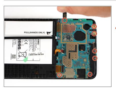
Remove the seven 4mm PH000 screws holding the motherboard in place.
