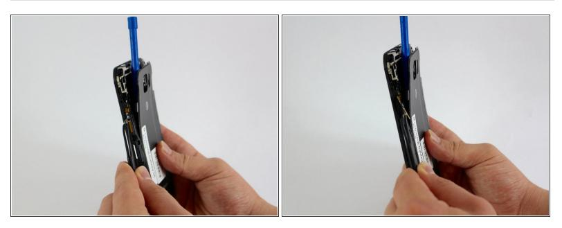
Use the tweezers to pry up the power button ribbon cable until the only thing attached to the frame are the contacts.
