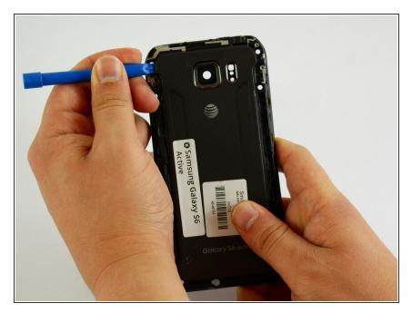
Insert a plastic tool between the frame of the phone and the back cover at the top left corner.
