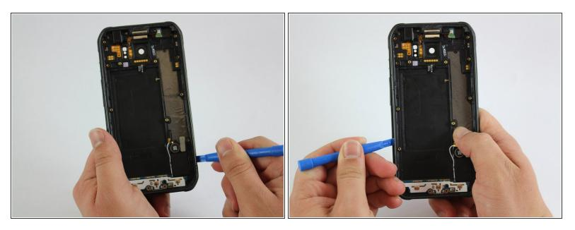
Once you see a large enough gap, insert a plastic tool between the frame and the plastic cover and slide it around the phone to separate both components.
