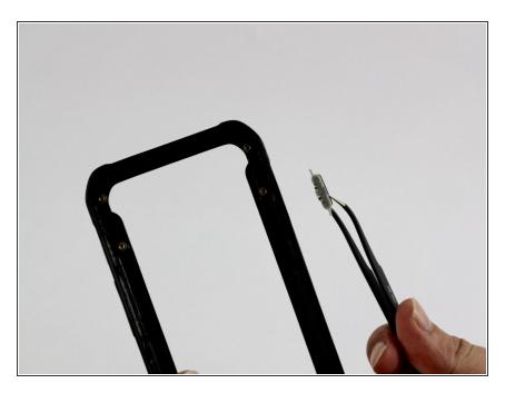
• Remove the power button from the frame.
