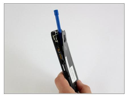
Leave the plastic tool inside in order to access the power button connection.
