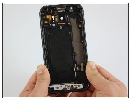
Put a little pressure on the top, on the bottom, and on the sides of the phone to separate it from the plastic cover.
