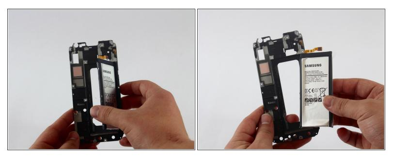
• Remove the battery from the frame.
