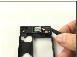
Flip over the black back cover and locate the speaker phone at the bottom, then use the tweezers to remove the speaker. It is glued to the back cover so a little force will be needed.
