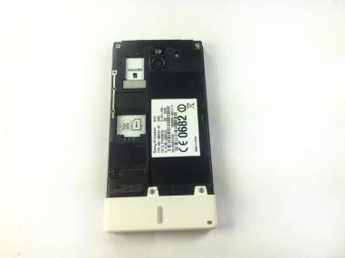
Push the back cover as shown, then lift the cover off.
