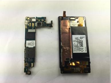
After removing all connectors, Use the plastic opening tool to slide it under the top left of the board then lift the board straight up.
