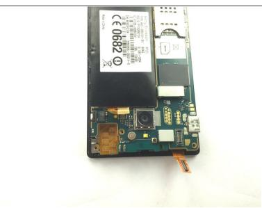
Repeat the last step as shown to remove additional power circuit which is on the top of the battery.
