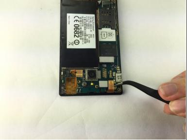
• Lay the phone down as shown. Then use tweezers to pull additional power circuit up gently to remove it as shown.
