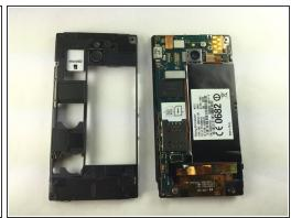
Turn the phone onto its side and insert a flat object and gently remove cover, using plastic opening tool as shown.
