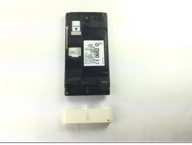
Use plastic opening tool to remove the bottom white cover as shown.
