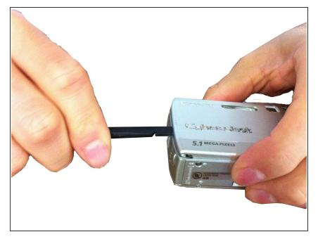
• Using a spudger, carefully pry open the front casing.
