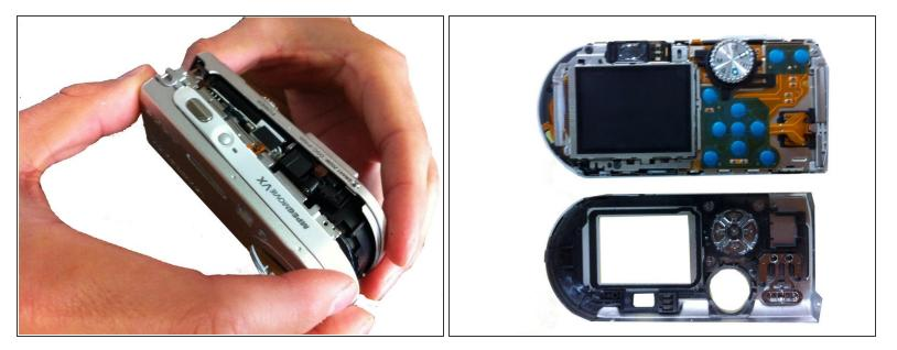
• Carefully pull the back casing away from the camera.
