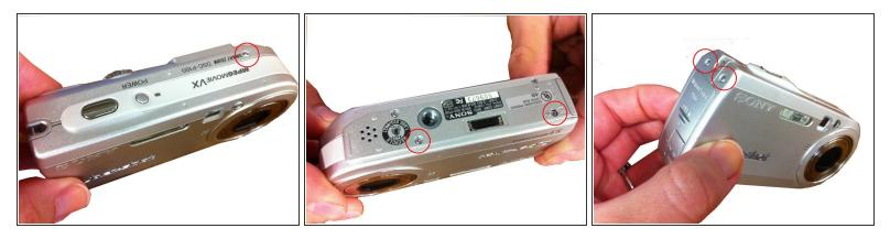
• First locate the appropriate screws for detachment.
