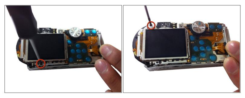
• Remove the two screws on the back side of the camera surrounding the LCD screen.
