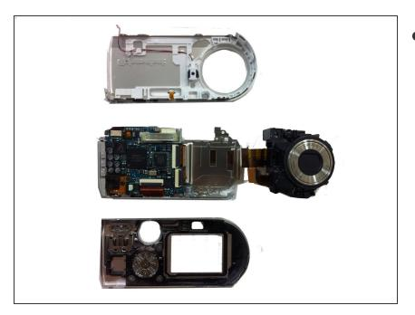
• The lens is now successfully removed from the camera.
