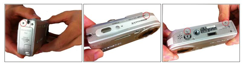
• Remove the four screws from the casing.
