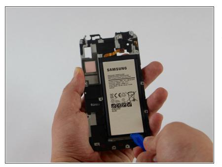
Insert a plastic opening tool on the side of the frame and pull out the battery.
