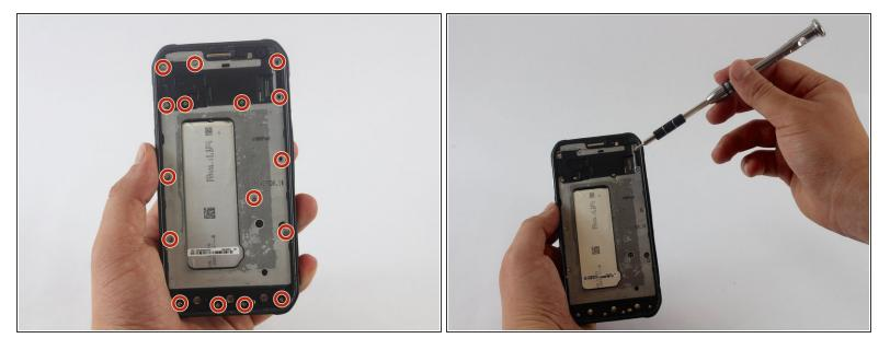
• Use the Phillips Head Screwdriver sized PH000 to remove the sixteen 4mm screws from the frame.
