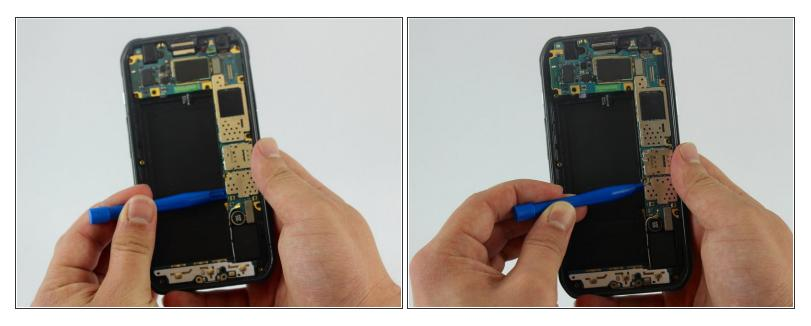
• Insert the flats end of the spudger below the motherboard and twist it to pry the board up.
