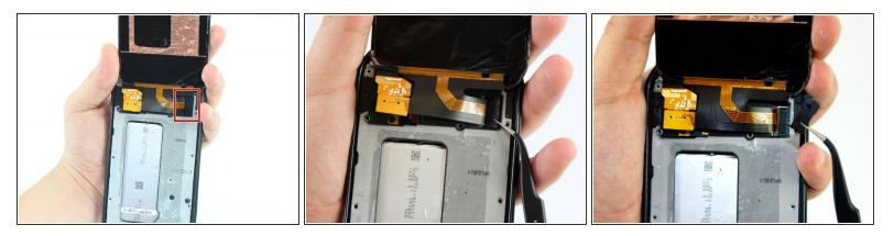
• Once the glass is off, you will see a small clip covering the screen connection to the motherboard at the top of the phone. Use tweezers to grab the clip by the crease on its side and pull it out.
