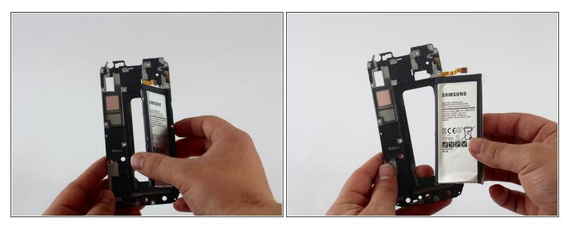
• Remove the battery from the frame.
