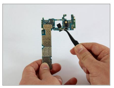
• Use the tweezers to remove the front camera from the motherboard.
