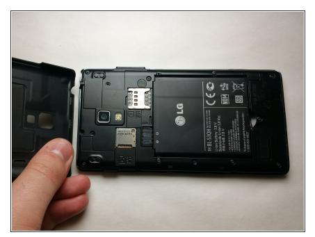
Power off the device and gently lift the battery cover off to access the battery
