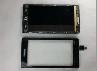
Carefully remove the digitizer from case by sliding out connected ribbon cable
