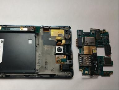
Gently lift the motherboard with small prying tool to remove and set aside
