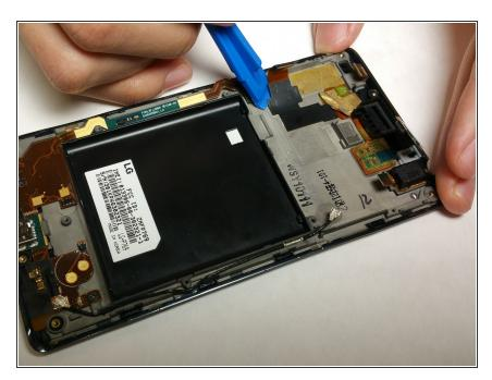
Use a small prying tool to detach the screen circuitry from the case
