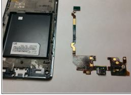
Use a small prying tool to detach the Micro-USB circuitry from the case of the phone
