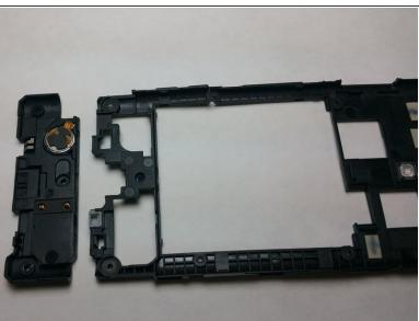
Carefully remove vibration and speaker module using the prying tool
