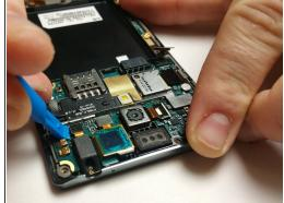
• Use a small prying tool to release all motherboard connections.
