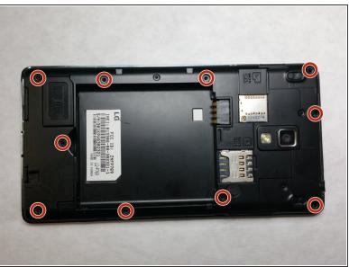
Remove all 10 of the 4.5mm screws that hold the back frame to the case of the phone using the PH000 headtype
