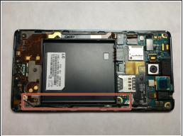
Remove both connections of the antenna by pulling up with tweezers
