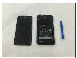
Using a plastic opening tool, take off the back cover of the phone.
