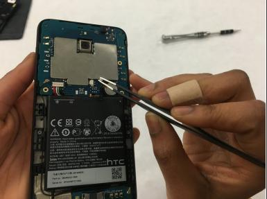
Pull the wire harness from the circuit board that is connected to the vibration motor using a pair of precision tweezers.
