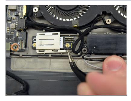
Using the tweezers, lift up on the retaining tab of the module retention bracket and slide the bracket to the left, then lift it free.
