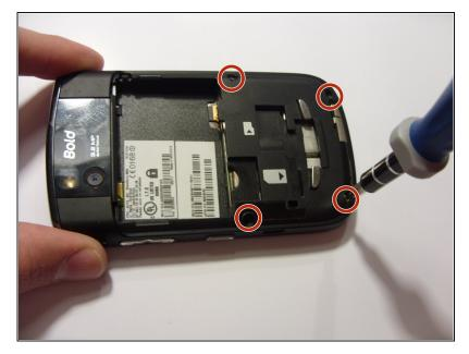
Using a T6 Torx screwdriver, remove the four screws from the bottom half of the device.
