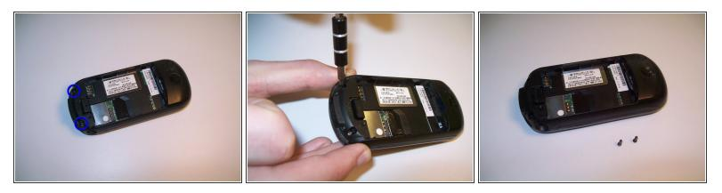
• Use a Torx T-5 screwdriver to remove the screws on the back of the phone.
