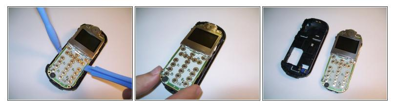
• Use plastic opening tools to free the circuit board from the case.
