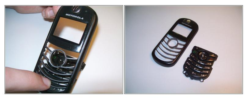
• On the top half of the phone push downwards on the number keys to free the keypad from the top of the phone.
