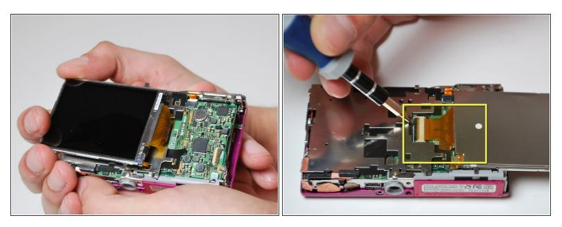
• Pull the LCD screen to the left slightly, lift it and flip it open to the right.
