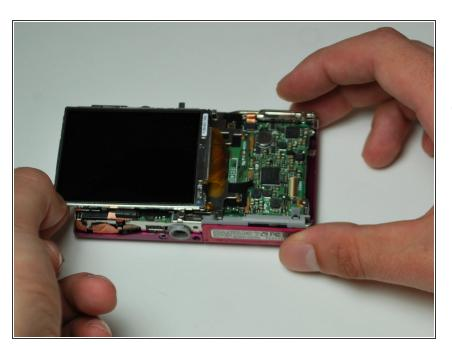
Using your index finger, guide the cable of the new screen into place.
