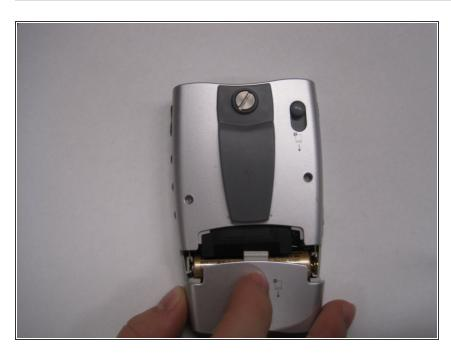
Using your thumb, slide down and remove the battery cover.
