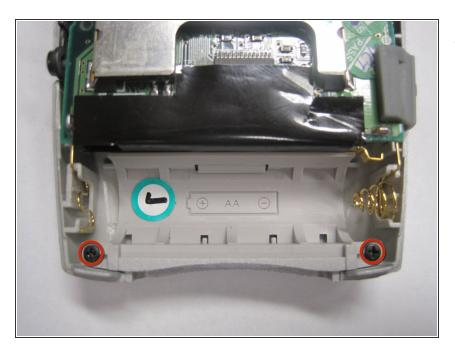
Using a Phillips #00 Screwdriver, remove the two 5.5mm screws from the sides of the battery compartment.
