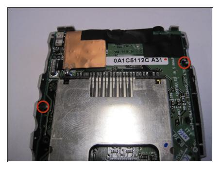
Using a Phillips #00 Screwdriver, remove the two 5.5mm screws on the left and right edges of the circuit board.
