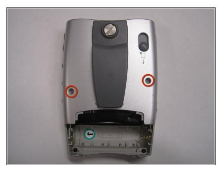
Using a Phillips #00 Screwdriver, remove the two 7.5mm screws from the sides of the back cover.
