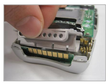
Carefully remove the battery compartment.
