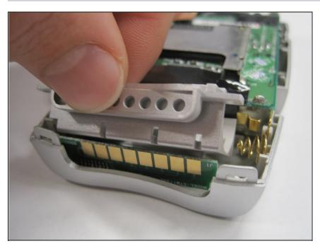
• Carefully remove the battery compartment.
