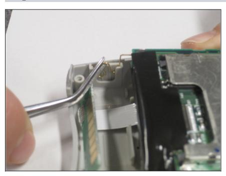
Using a pair of tweezers, carefully pry the metal loop on the left side of the battery compartment away from the case.
