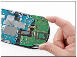
Starting from the upper left corner, use a spudger to pry up and remove the left button board.
