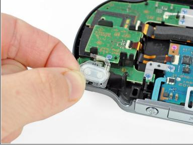
Using a spudger, gently peel up the left shoulder button from the light adhesive connecting it to casing.
