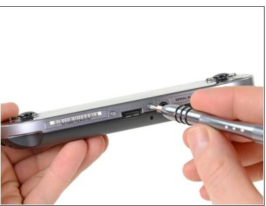
Remove the two 5.4mm Phillips #00 screws on the bottom of the device near the charging port.
