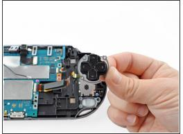
Using tweezers, peel up and remove the directional pad.
