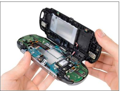
Gently separate the two cases, minding the battery and the touch screen controller connectors holding the two cases together.
