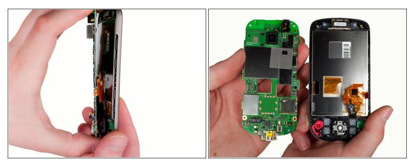
• Gently lift the motherboard out of the front enclosure once the screws are removed.
