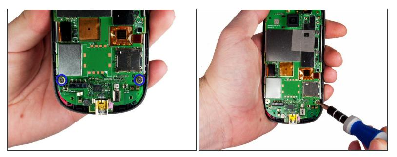
Remove the two screws located at the bottom left and right of the motherboard using a small Phillips screwdriver.
