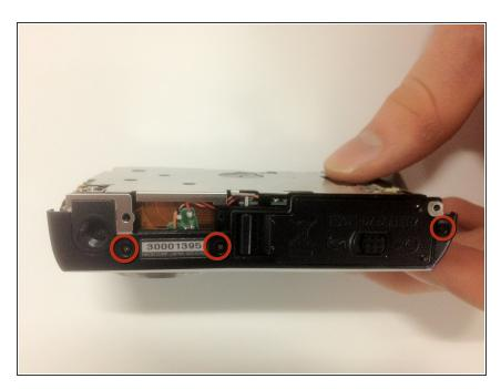
Remove the three 3x3mm screws that attach the front casing to the bottom.
