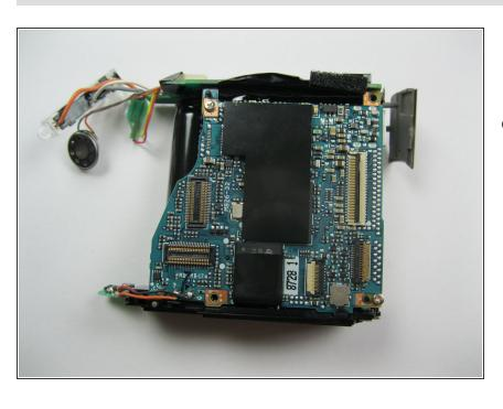
Once the lens assembly has been removed, the mother board cannot be disassembled any further. To reassemble your device, follow these instructions in reverse order.
