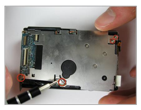
Remove the two 3x2 screws and two 3.5x2.5 screws attaching the rear panel to the motherboard.
