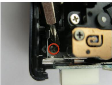
Remove the final 4x3mm screw at the top of the camera near the lens.
