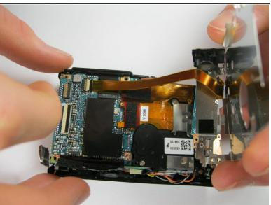
Lift the back panel off the motherboard.
