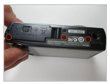
Remove the three 3x3mm screws attached to the rear casing.
