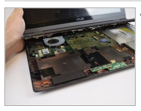
Carefully lift and remove the plastic cover to avoid damaging anything.
