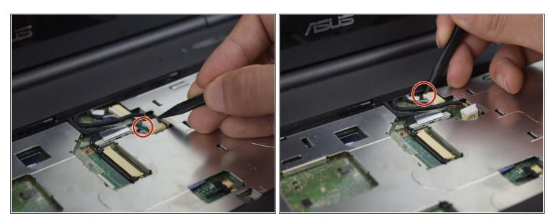
Use the spudger tool to unplug the two cords from the body by pushing on the tabs on both sides
