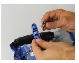
Pull the charging port mount away from the housing. Once separated, pull the the charging port out
