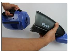
Remove the dust cup container from the motor housing.
