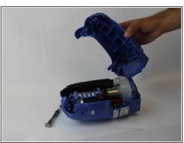
Remove the five 14mm screws with the PH 2 bit. Once all the screws are removed, pull one part of the housing away from the other.
