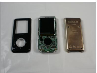
Pull the front cover away from the rest of the device.
