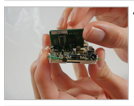
Carefully peel the memory board away from the rest of the motherboard
