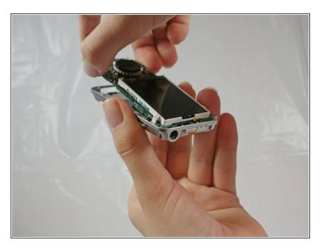
Pull the bottom of the motherboard up and then out.
