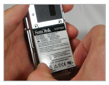
Grip the bottom of the battery with your thumb and forefinger and pull it away from the device.
