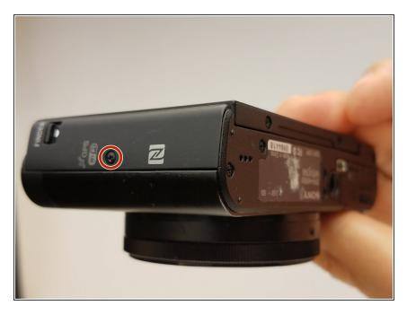
Remove the marked screw on the side of the camera with a Phillips #000 screwdriver.
