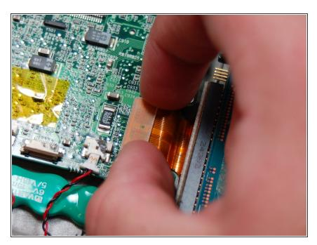
Carefully pull up on the hard molded plastic portion of the ribbon to detach it from the computer.
