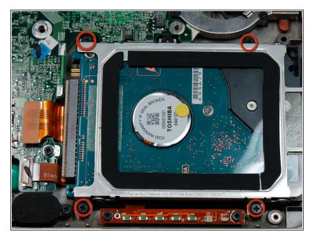
Remove the 4 #00 5 mm screws holding the hard drive to the case.
