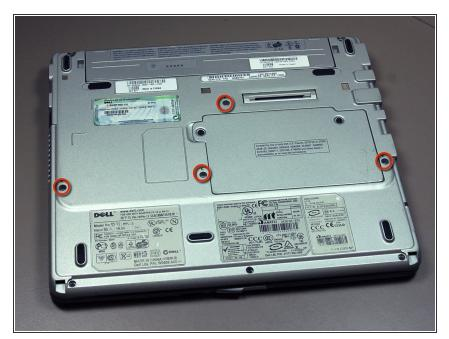
Remove the four 4 mm Phillips #0 screws from the bottom of the laptop.
