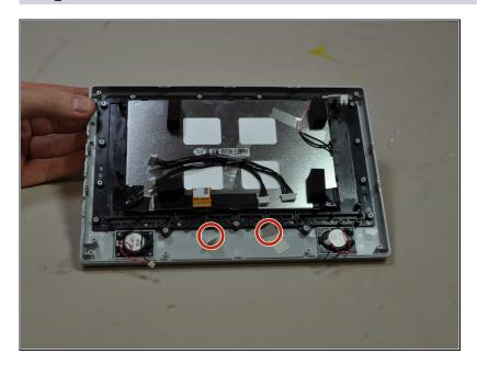
Peel back the tape holding the button clusters down.
