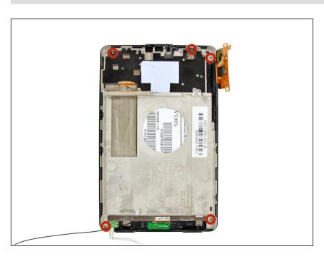
Remove the five 3.6 mm Phillips #00 screws securing the frame and ambient light sensor.
