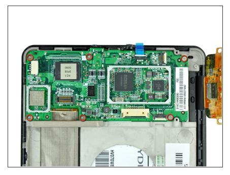
Remove the six 2.6 mm Phillips #00 screws securing the motherboard to the frame.
