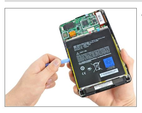
Repeat the process from the previous step to free the left battery cell.
