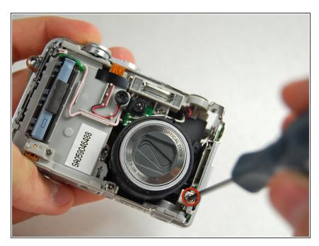
Remove the screw connecting the wifi card cover to the front of the camera.
