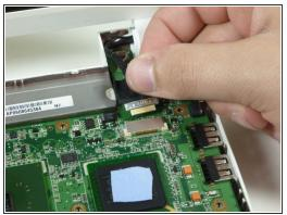
Remove the large black wire using a plastic opening tool.
