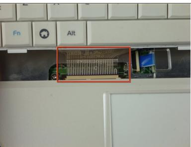
Clips hold the bottom portion of the keyboard to the laptop. Gently lift the upper portion of the keyboard and then move the entire keyboard towards the computer's screen until the ribbon cable is visible.
