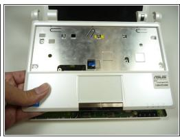
**Caution:** To clear the audio and microphone, lift the right half and move the cover to the left (as shown in the second picture) to prevent cover damage.
