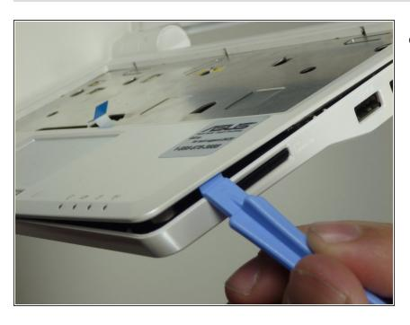
Use a plastic opening tool to gently detach the top cover from the laptop's base. See the next step for removing the cover.
