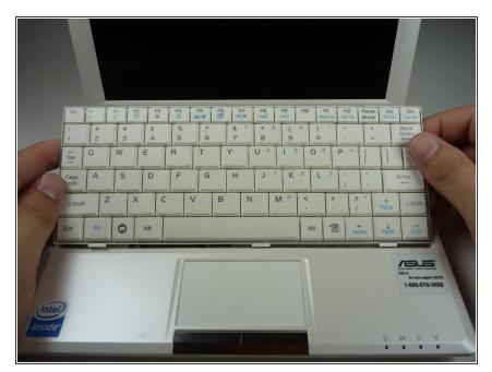
Remove the keyboard by lifting upwards.
