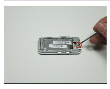
Remove the single 0.327" silver screw on the back of the device that was exposed when you removed the rear case cover.
