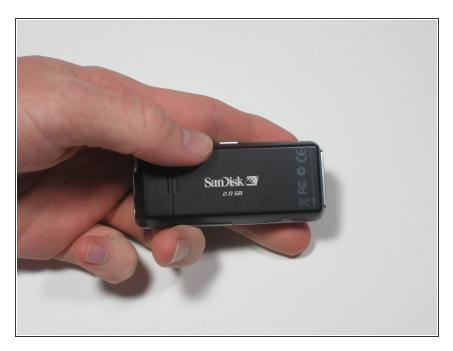
Slide the back cover forward toward the top of the device with your thumb.
