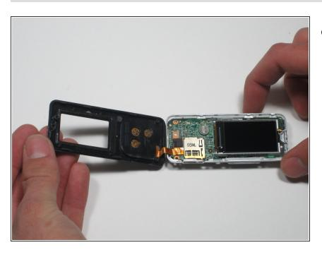
Open the case cover starting on the side most distance from the buttons.
