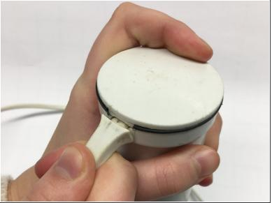
Pull back the rubberish part of the power cord, located at and connected to the top of the mixer
