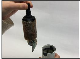
Take out motor and circuitboard by pulling the rotational cylindric part upwards.
