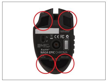
Using a spudger, remove the teflon tape on the bottom of the mouse to reveal four screws.
