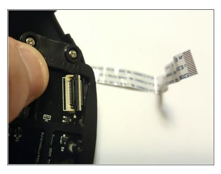
Gently pull the white connection strip out of both connection ports.
