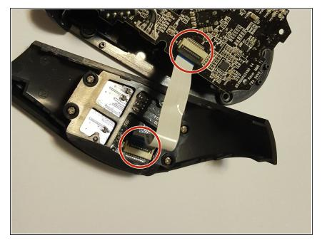
Flip open the black pieces on either end of the white connection strip holding the side buttons onto the circuit board.
