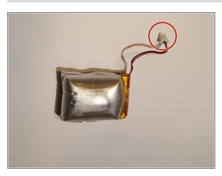
Unplug the power cord from the circuit board in the mouse.
