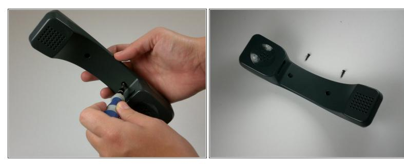
Unscrew the two black screws (8 mm long) located in the middle of the handset using #1 Phillips head.
