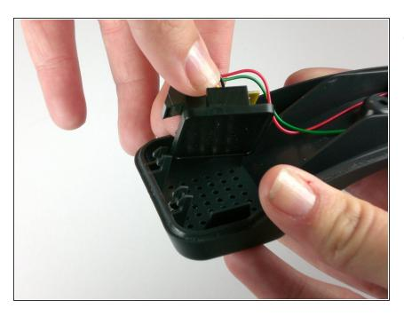
While holding the handset front cover, grasp and twist the handset microphone and jack until they come free from the cover.
