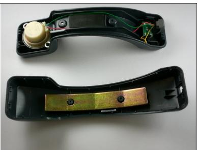
Pry the back cover off the headset using a spudger. It is best to pry at the top of the handset.
