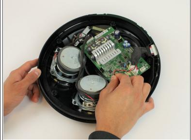
• Disconnect the two pressure connections from the circuit board.
