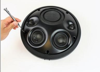
Remove the five 14.4 mm T10 Torx screws.
