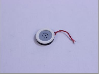
Replace the broken speaker of the phone and solder it back in place.
