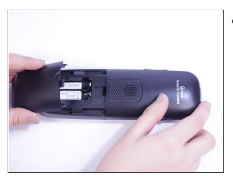
Lift out both batteries with a prying movement.
