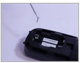
Remove the following two Phillips #00 screws securing the back casing to the front.
