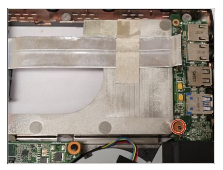
Remove one (1) 5mm x 4mm screw with the size 0 Phillips head screwdriver.
