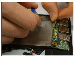
Pull up on the black ribbon connection on the audio board. The board will lift out of the device casting.
