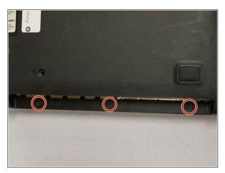
Remove three (3) 3mm x 3mm screws with the size 0 Phillips head screwdriver.
