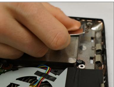
Using both hands pull the audio board out by pulling towards the center of the device and then up to remove.
